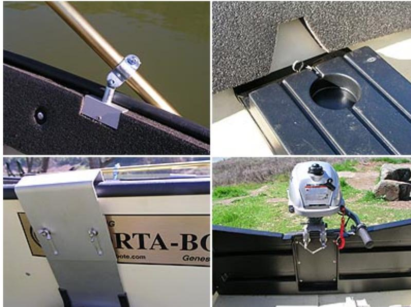
[Top left] The oar mounts are built onto the side of the boat. [Top right] The cup holders on the seat provides a solid place to put your beverage. [Bottom left] The top portion of the Porta-Dolly hooks easily onto the boat. [Bottom right] A solid plastic transom provides a strong place to mount the motor
