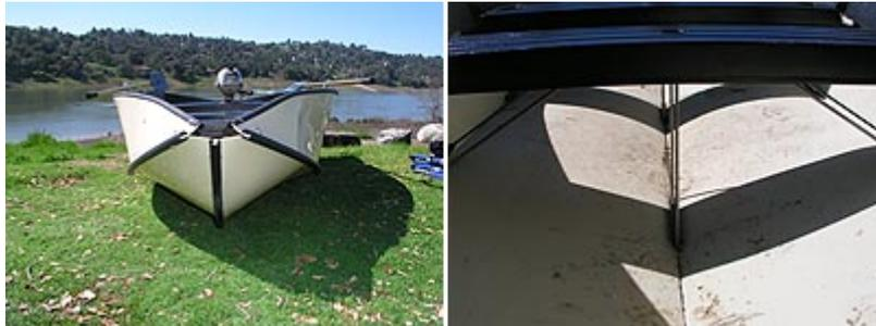
A deep entry V-hull provides good hydrodynamics in the water. The picture to the right shows the floor that's flexible and yet stable
