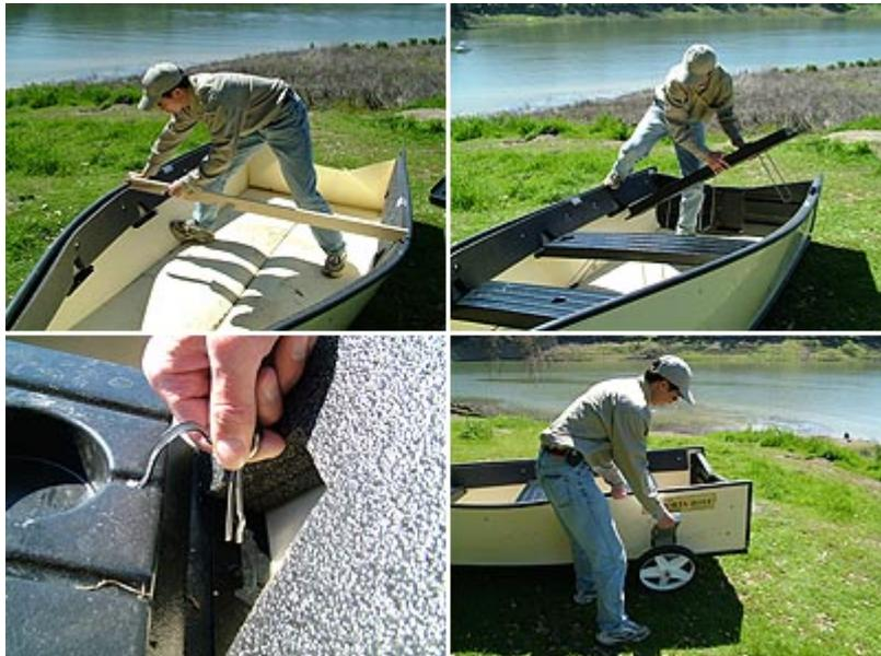
Setting up the Porta-Bote takes just a few minutes. Everything snaps into place then is secured either via cottle pins or nuts, bolts, and washers
